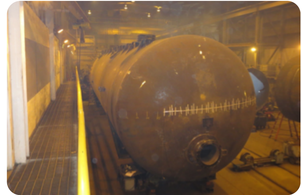
Horizontal Spray Deaerator Capacity: 2,000,000 lb/hr Not Recommended for Higher Capacity Power Plants
